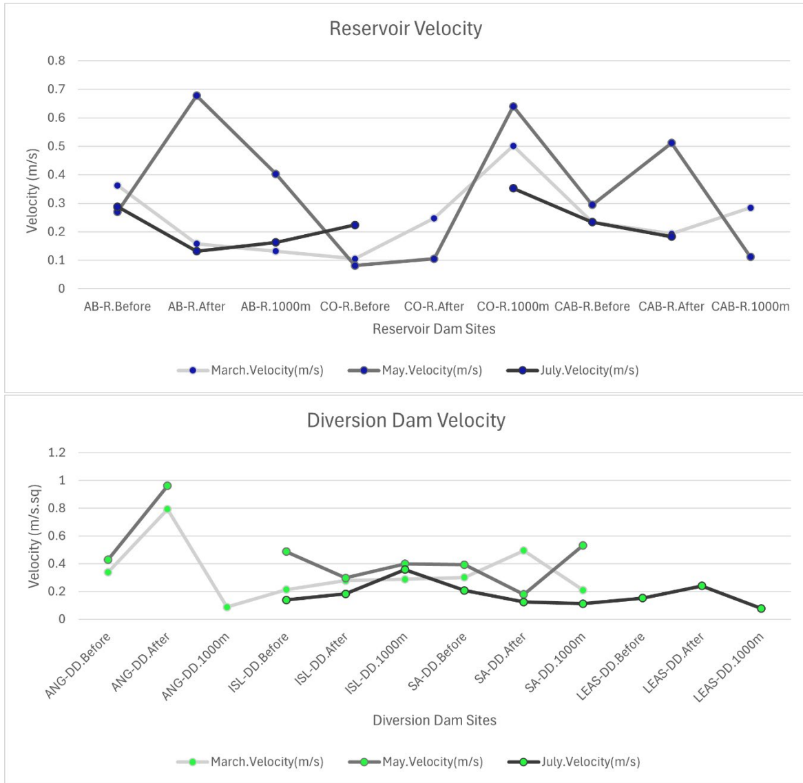
Figure 5. Comparison of average velocity (m/s) for Reservoirs and Diversion Dams for each measured sampling period (March, May, and July)
